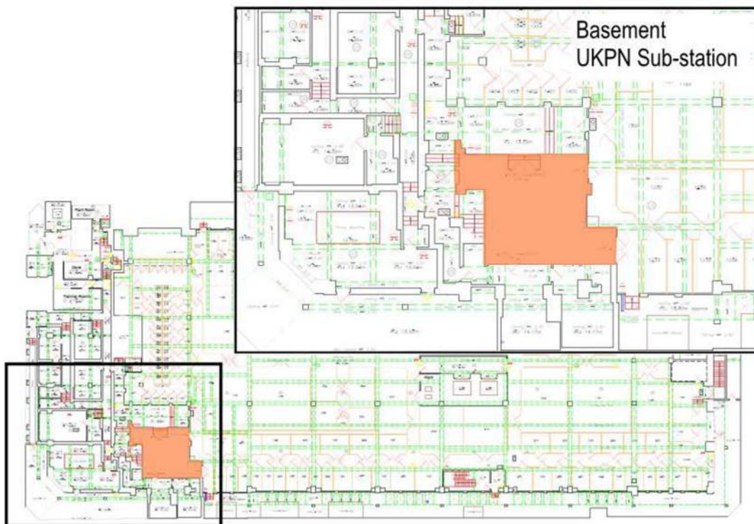
Extract of UKPN plan denoting existing sub-station
