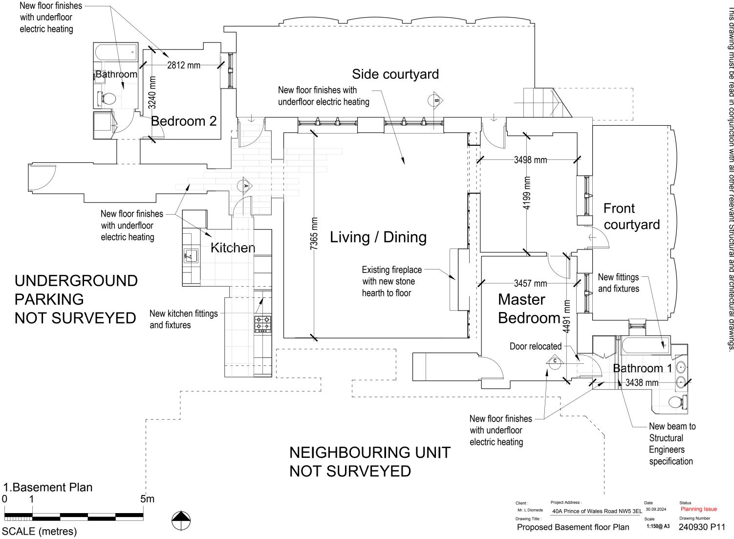
GENERAL NOTES: All dimensions and setting o This drawing must be read i out must be checked on site. in conjunction with all other relevant Structural and architectural drawings
