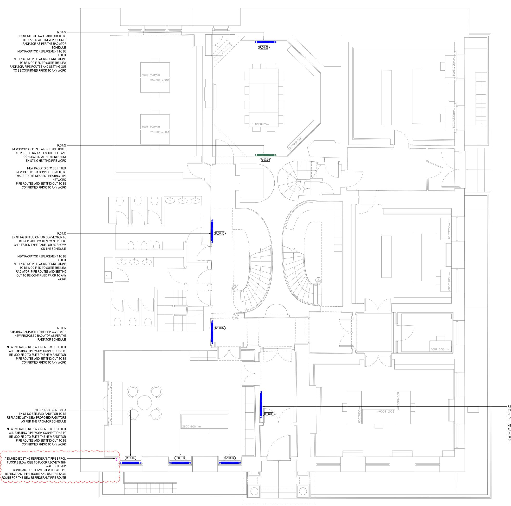
– R.00.06 EXISTING RADIATOR TO BE REPLACED WITH NEW PROPOSED RADIATOR AS PER THE RADIATOR SCHEDULE.
