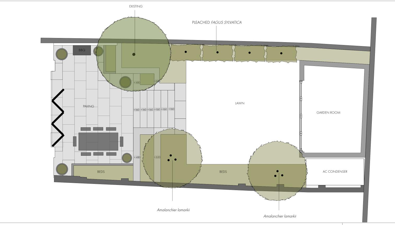
Terrace to be paved in sawn york stone. Drawing shows paving slabs at 900 x 600mm.
