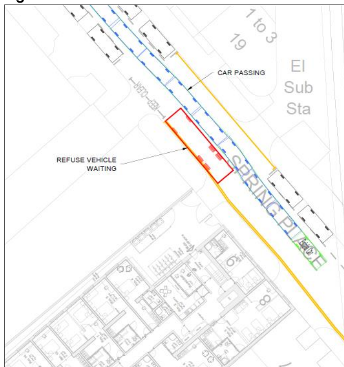
Figure 3A Locations for Refuse Collection and Delivery Vehicles to Stop
