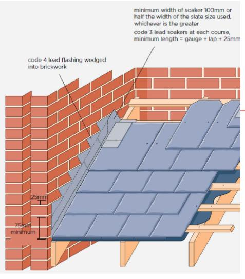
Typical detail at parapet abutment wall: Use slate and a half slate to form verge at parapet.
