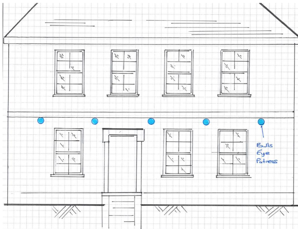
Fig (iii) – proposed positioning of pattress plates to the front elevation
