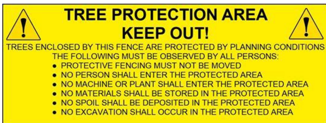
Fig. 4: Wording to be included in high visibility all-weather sign attached to protective fencing
