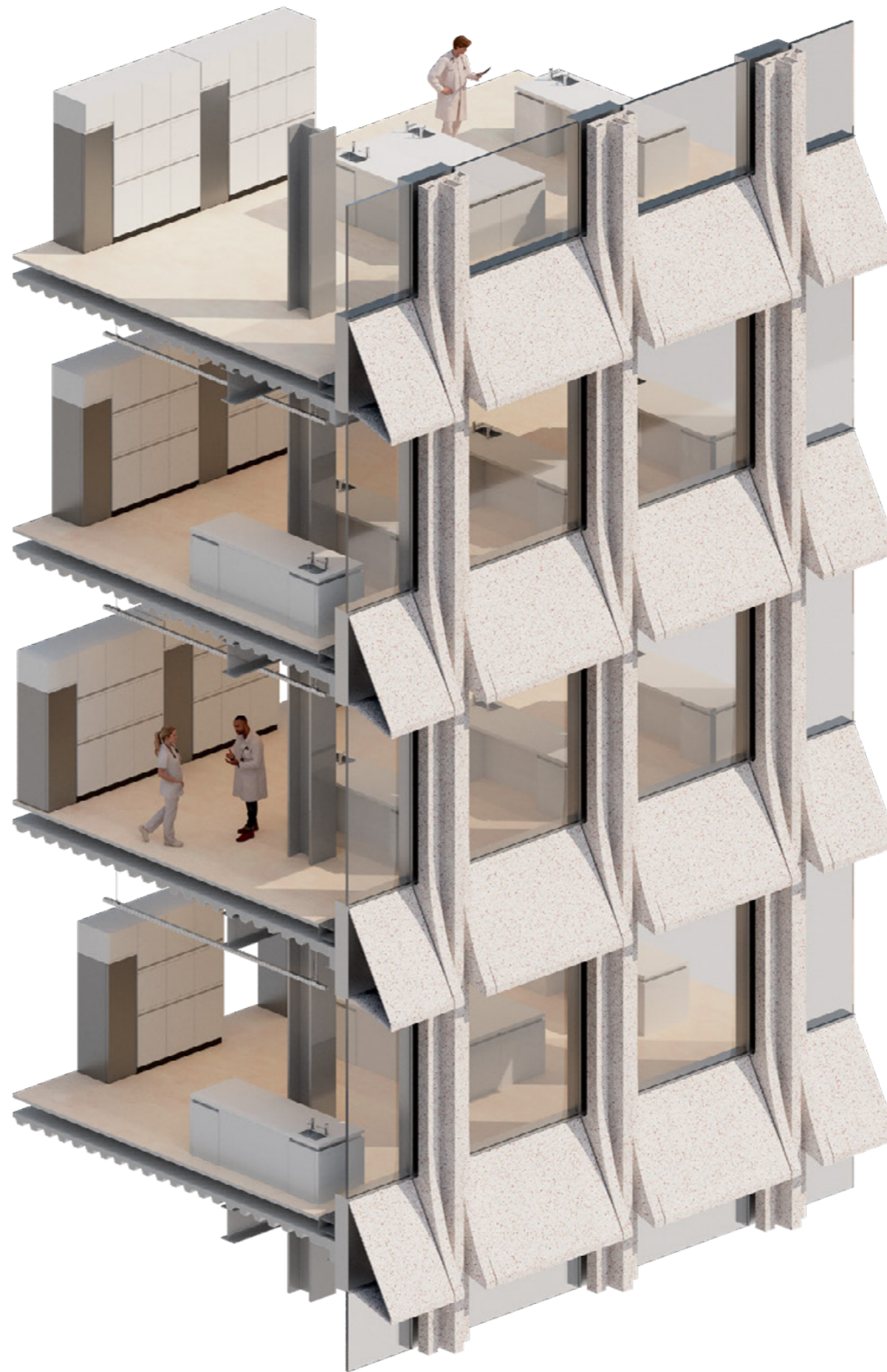
Diagram - Cutaway axonometric of lab-enabled tower facade
