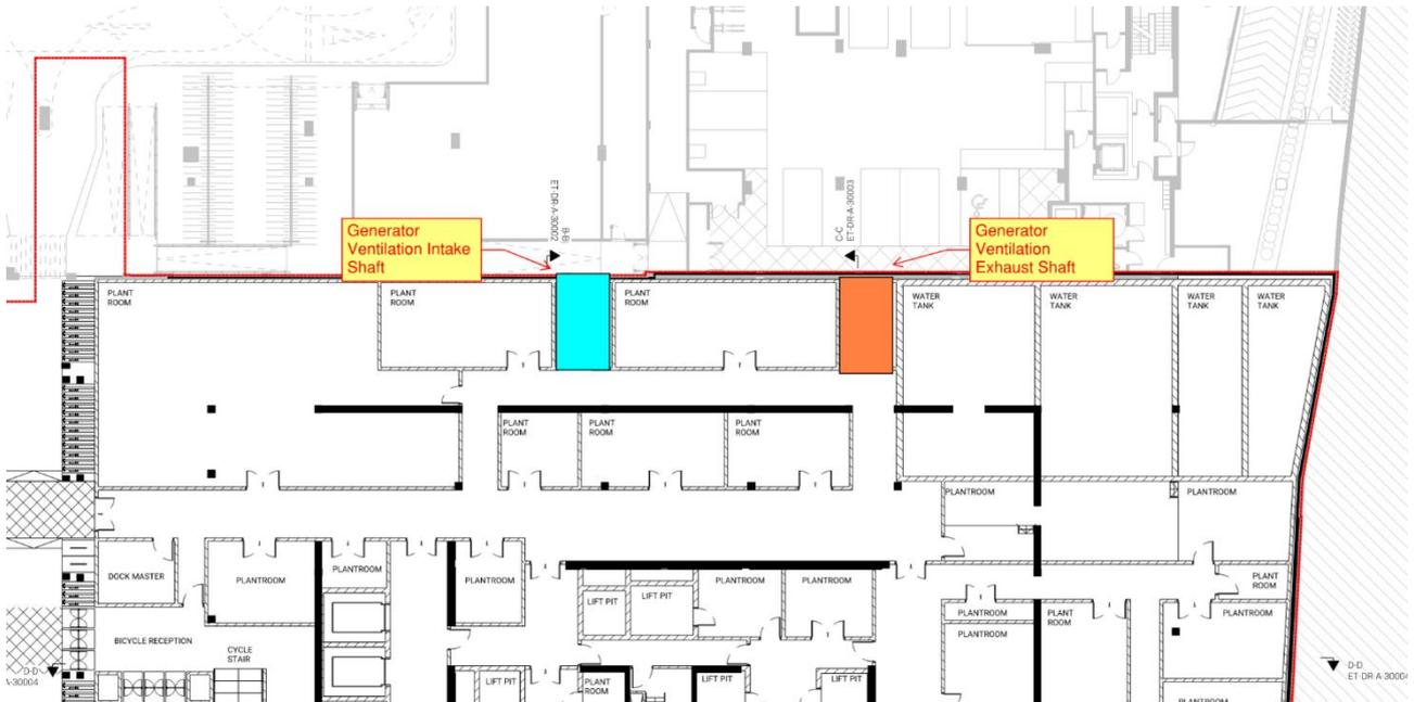
**Figure 10 – Image showing the generator plantroom location in the basement of Euston Tower**
