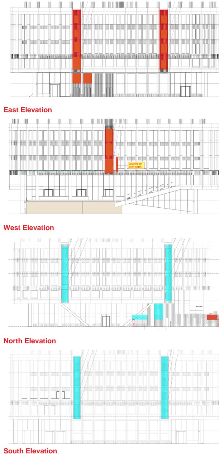
Figure 4 – Location of louvres on each elevation of the Podium (Exhaust in red, Intake in blue)
