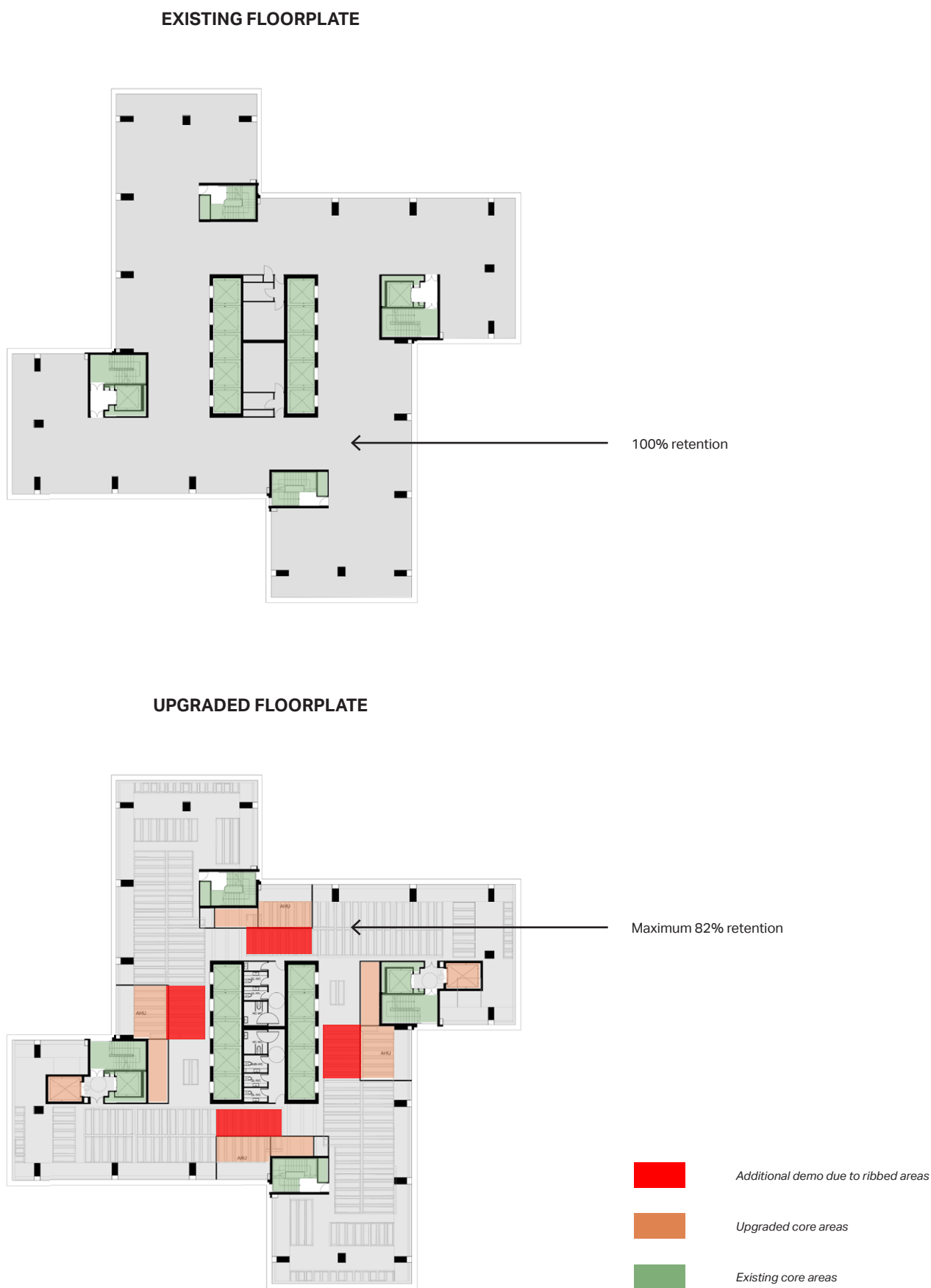
Figure 15.2 Diagram showing erosion of floor slab due to upgrades to meet current Building Regulations
