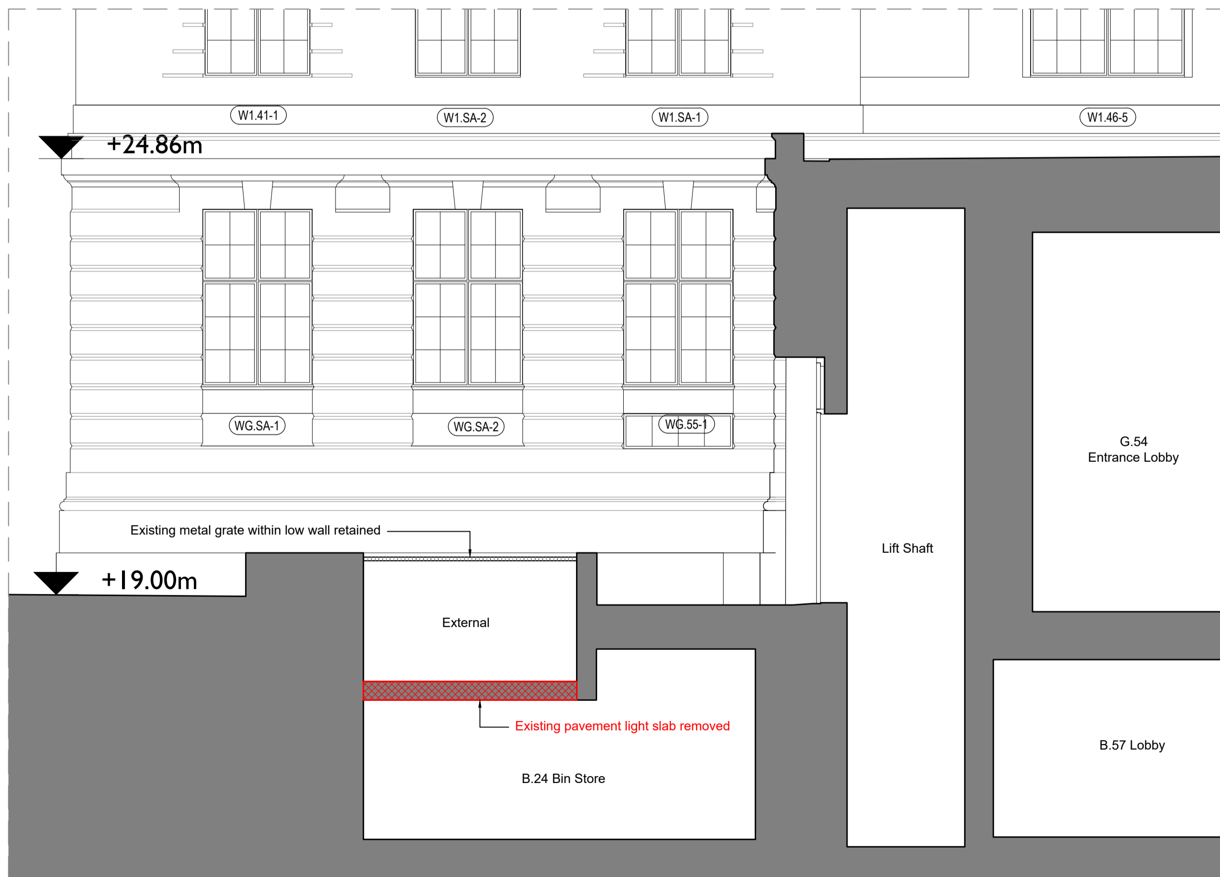
3 Existing section through pavement light showing demolition 2014 1:50
