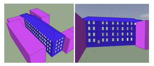
Images from thermal modelling software (purple blocks represent adjacent buildings, which provide natural shading)
