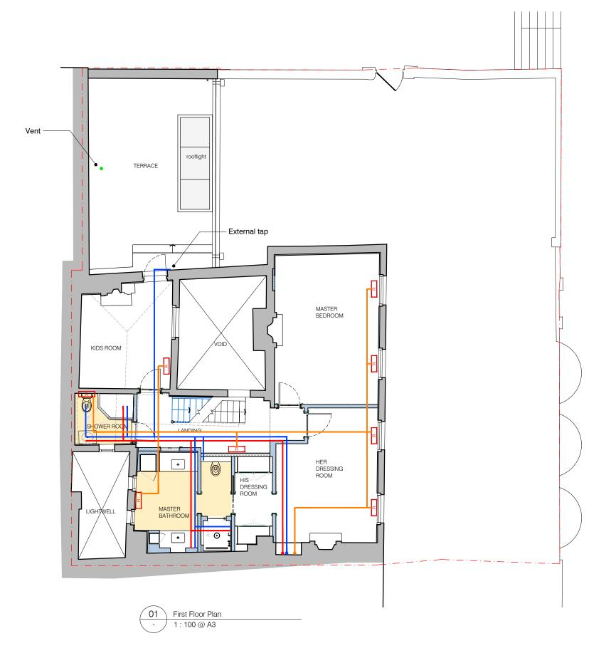
Services Key CU Consumer Unit gas Gas supply and meter elec Electric supply and meter water Water supply and meter Heating, flow and return routes --- Gas Cold Water --- Hot water Omitted ---- Vent/Flues Vertical services R Radiator Electric Underfloor Heating Wet Underfloor Heating Existing Inspection Chamber New Inspection Chamber (double sealed if internal) Sump Pump ----- Below ground sewage drainage
