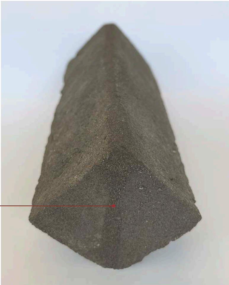
Brick aggregate dusted glued joint
