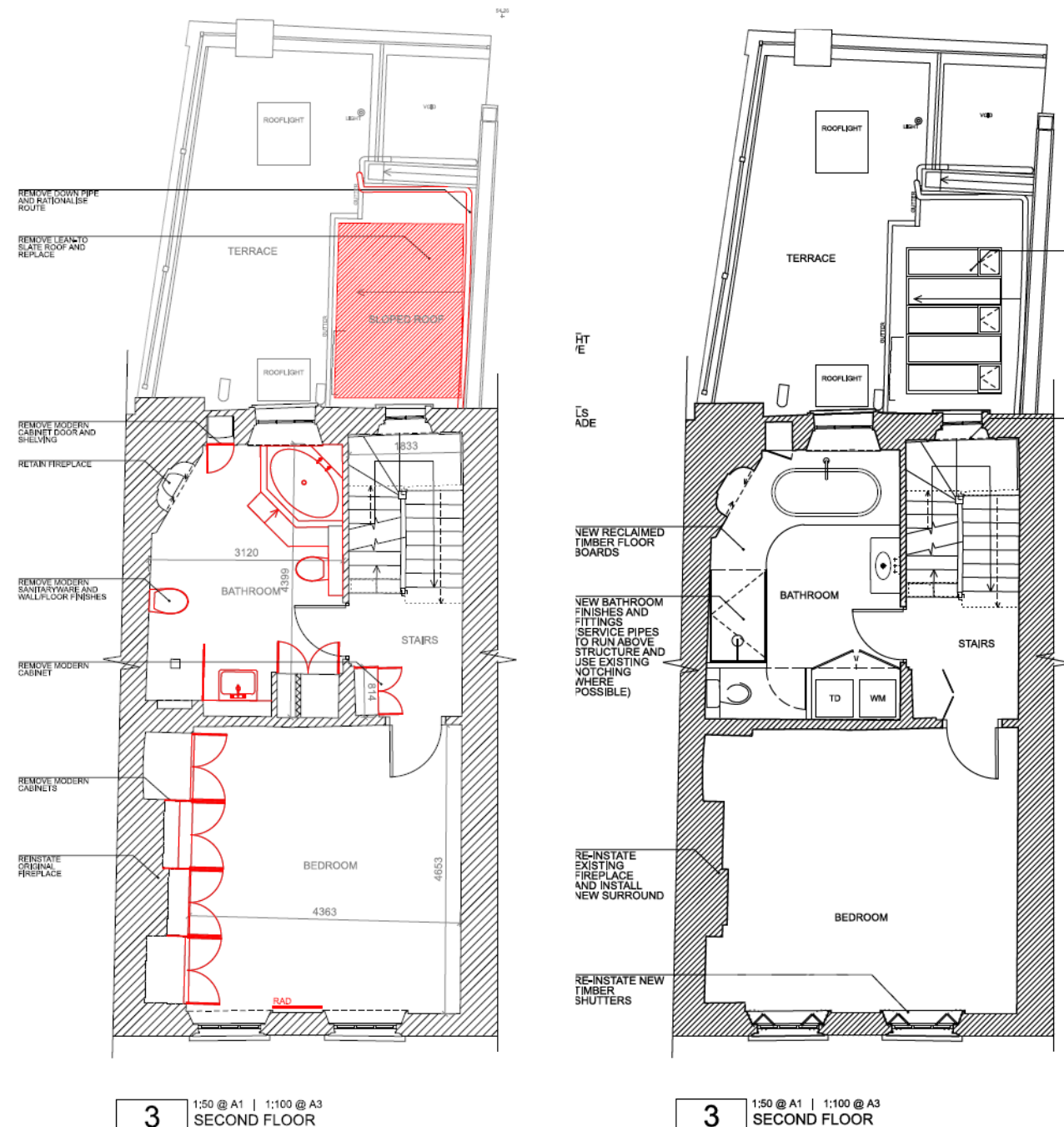
Figure 13: Second floor, existing/demolition and proposed plans.
