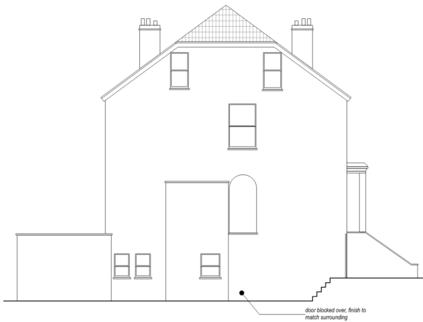
Fig 4. Proposed side elevation.
