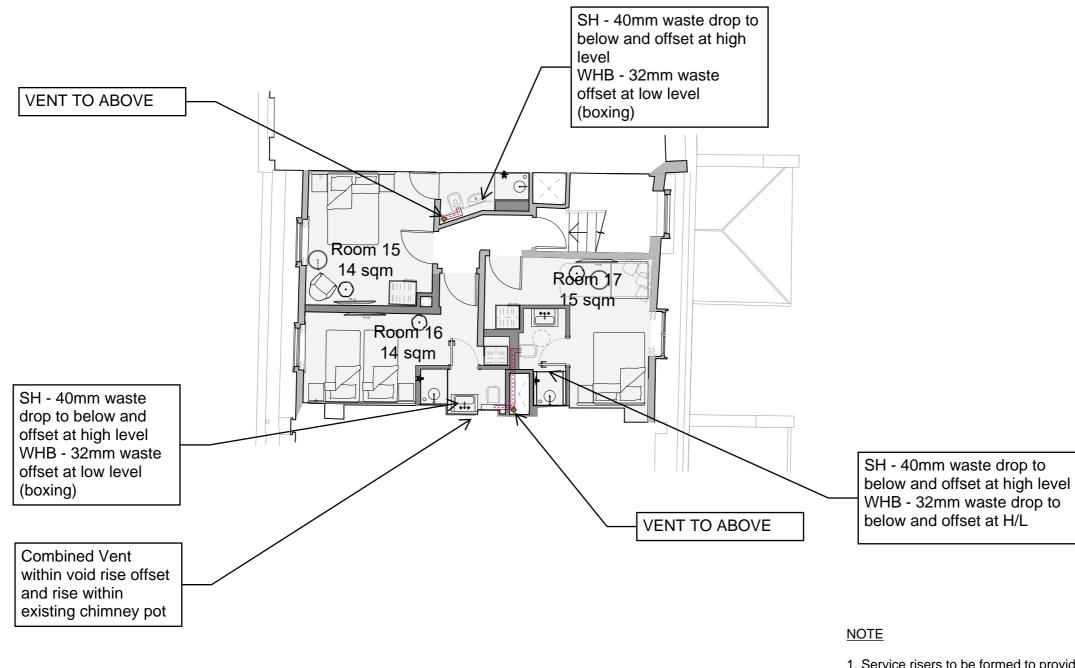
1. Service risers to be formed to provide concealed routing for ventilation ductwork and other services as part of the payout alteration work. Riser construction meet the performance requirements as set out within fire safety statement in order to resist the spread of between and floors and rooms.
