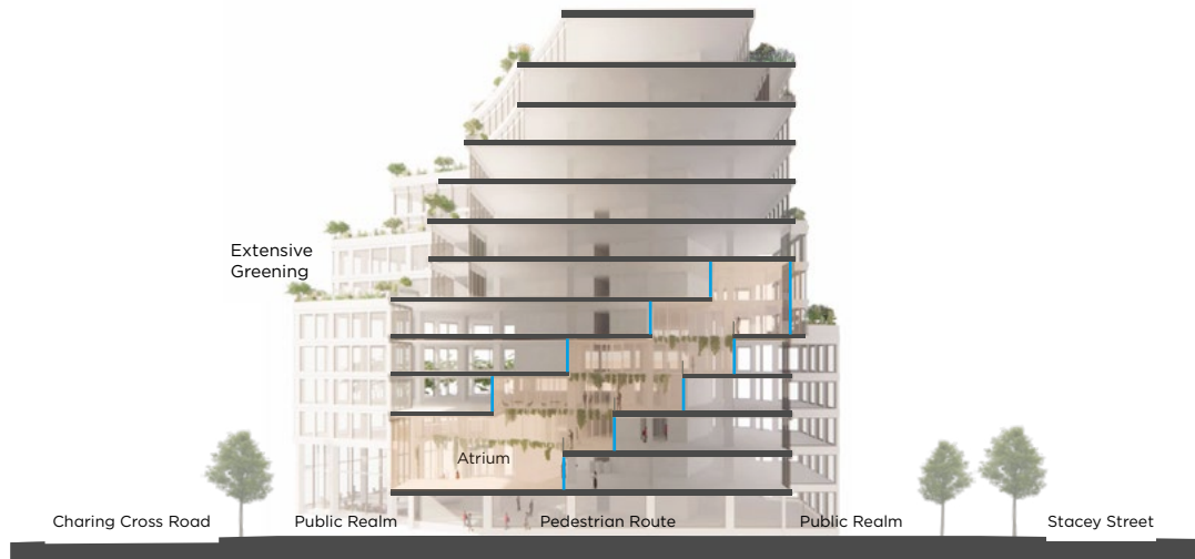
Proposed building section showing pedestrian walkway connecting Old Compton Street to New Compton Street
