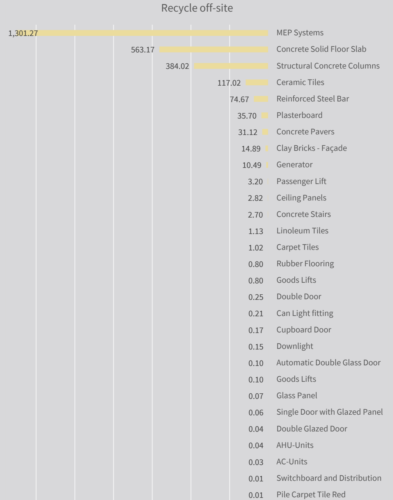
Figure 2-6 Materials by weight identified by Material Index as having potential for recycling
