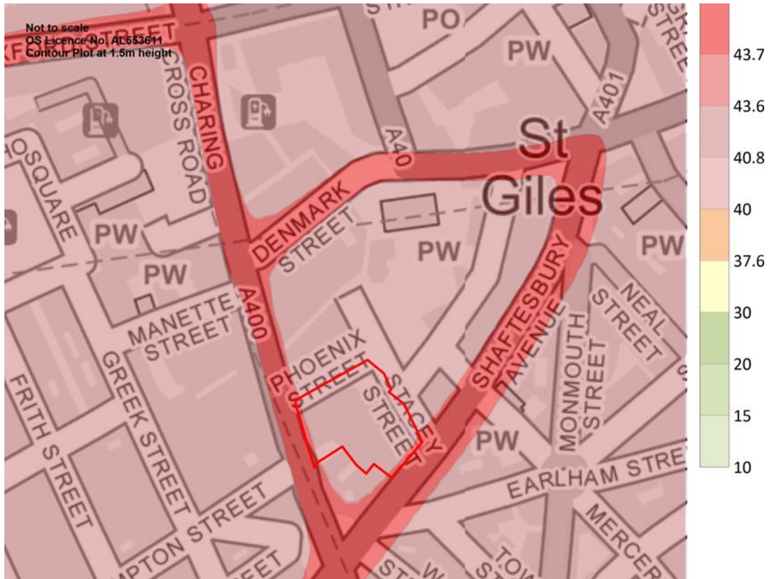
Figure 6-2. Total Long Term Annual Average Nitrogen Dioxide (NO 2 ) Concentration at Proposed Development ( \mu\text{g}/\text{m}^3 )
