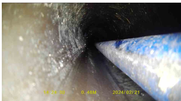
2b74d412-e0a8-464c-9e31-c12150a91c4c.jpg, 00:00:19, 0.48 m Other obstacles from 4 o'clock to 6 o'clock, 25%
