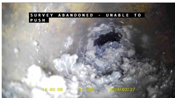
39ad9e52-f44f-45b2-a9b8-f6e2a4fa684d.jpg, 00:00:37, 0.19 m Survey abandoned, Camera unable to pass debris
