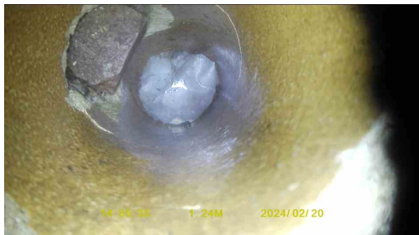
e20c5a1b-250b-45b3-8d80-c9757825fedf.jpg, 00:00:45, 1.24 m Other obstacles, protruding through wall from 9 o'clock to 11
