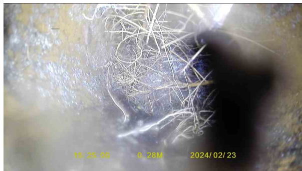
38ea1992-ce32-43af-82a8-5bfceb4d8b7c.jpg, 00:00:19, 0.28 m Roots, mass, 80% cross-sectional area loss, change
