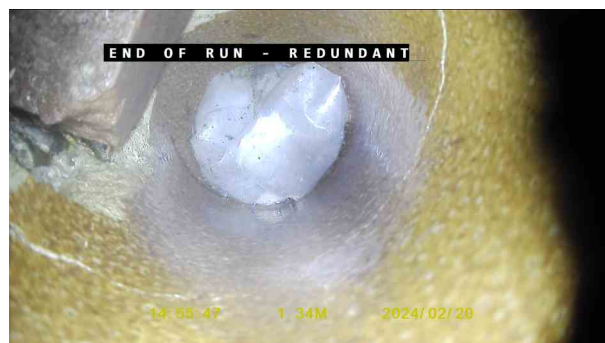
f70f8fbc-bf0e-473b-bf21-ad36d419e260.jpg, 00:00:51, 1.34 m Finish node, manhole, reference: Branch A, Redundant
