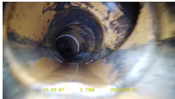
397b4b88-0e46-464b-87ce-6343e884bee4.jpg, 00:00:36, 2.78 m Junction at 2 o'clock, 100mm dia
