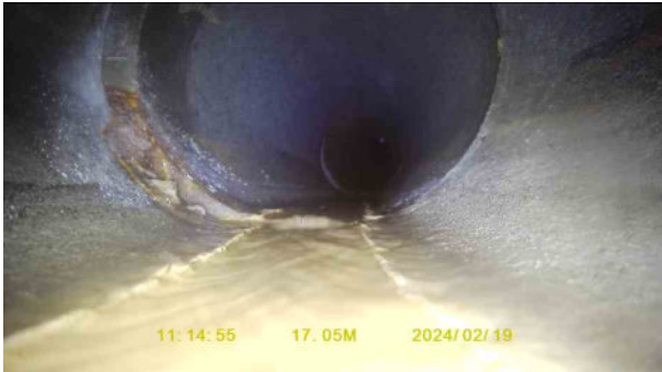
26c73e70-8711-4829-a15d-ed0453455f97.jpg, 00:03:02, 17.05 m Joint displaced, medium
