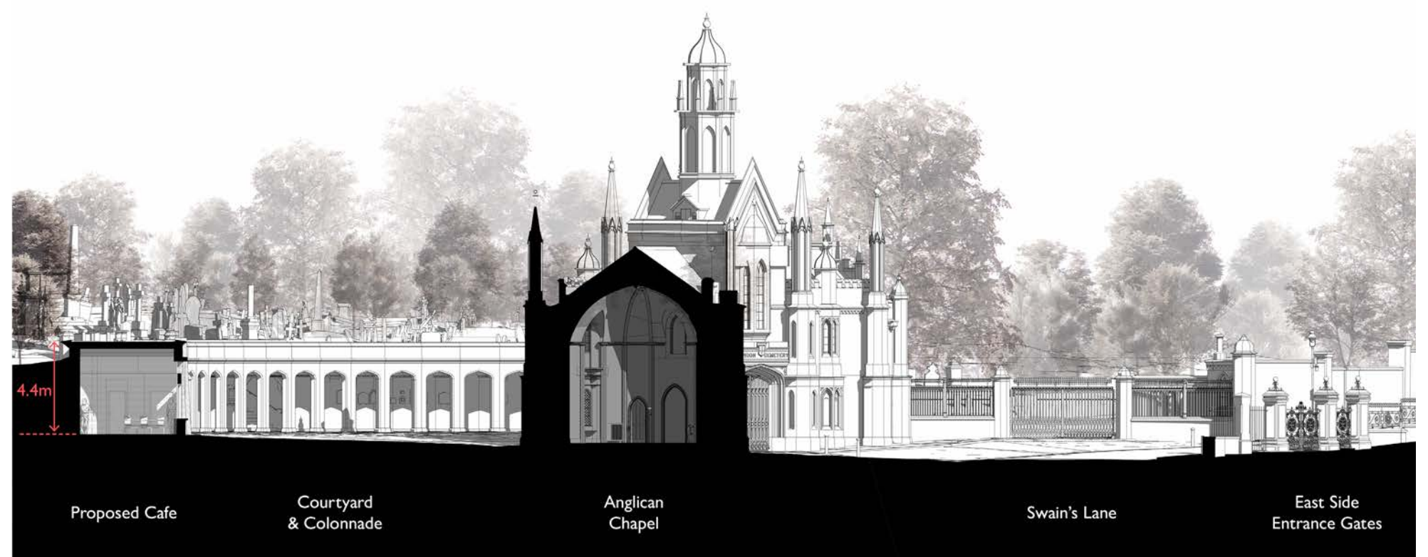
Section cutting through proposed cafe, showing its close spatial relationship to the Courtyard, Colonnade & Chapels.
