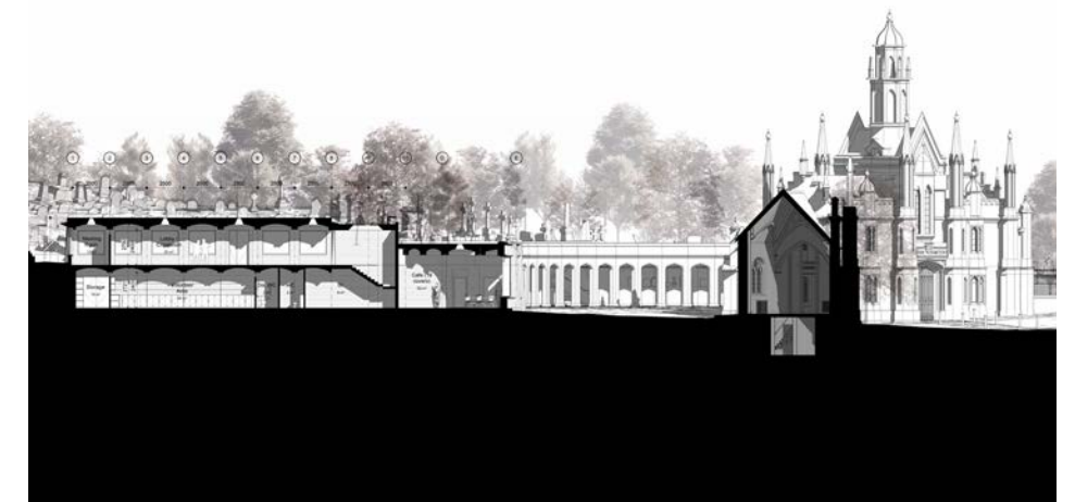
Concept Section showing the strategy to pop-up the massing away from the Courtyard.
