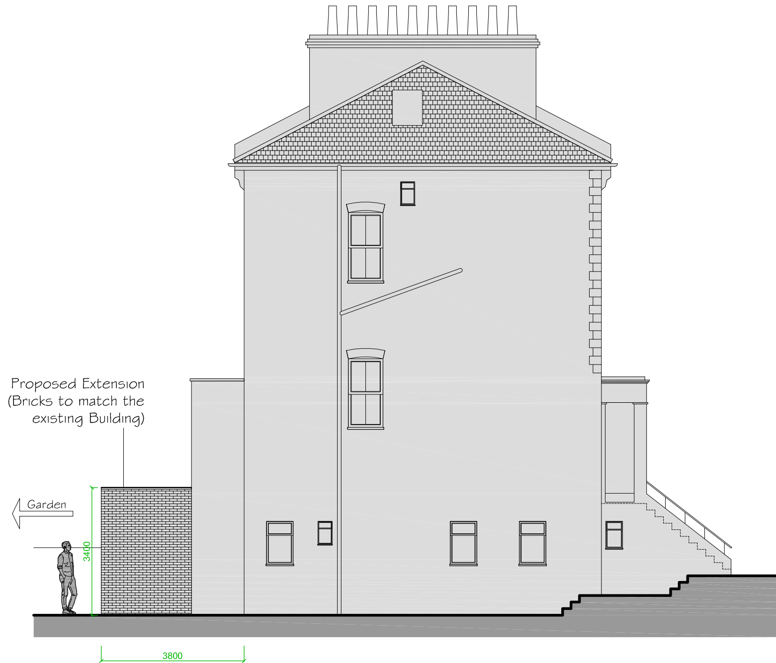
PROPOSED ELEVATION FROM THE SIDE OF No. 100 Scale: 1-100 @ A3
