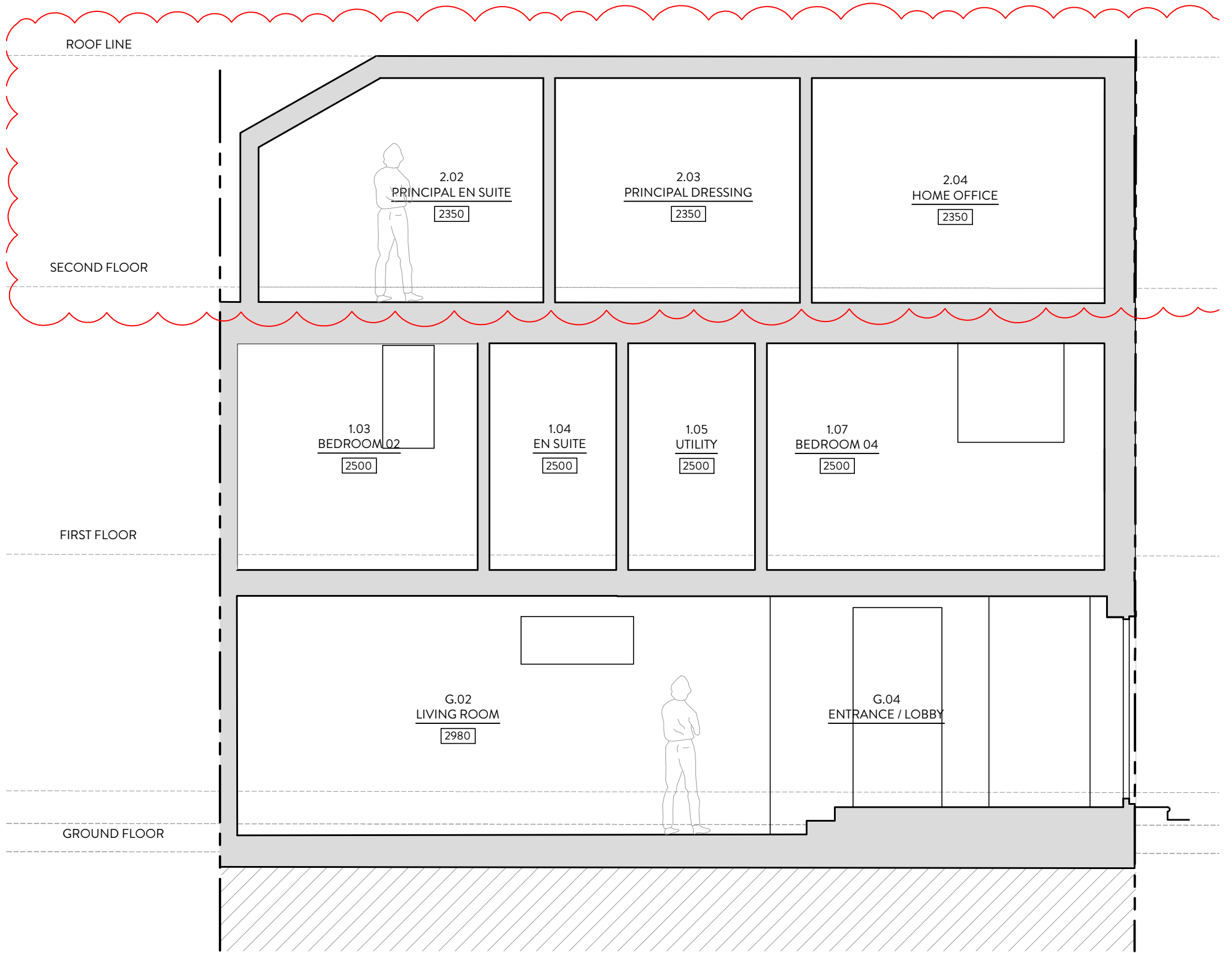
PROPOSED SECTION A-A @ 1:50
