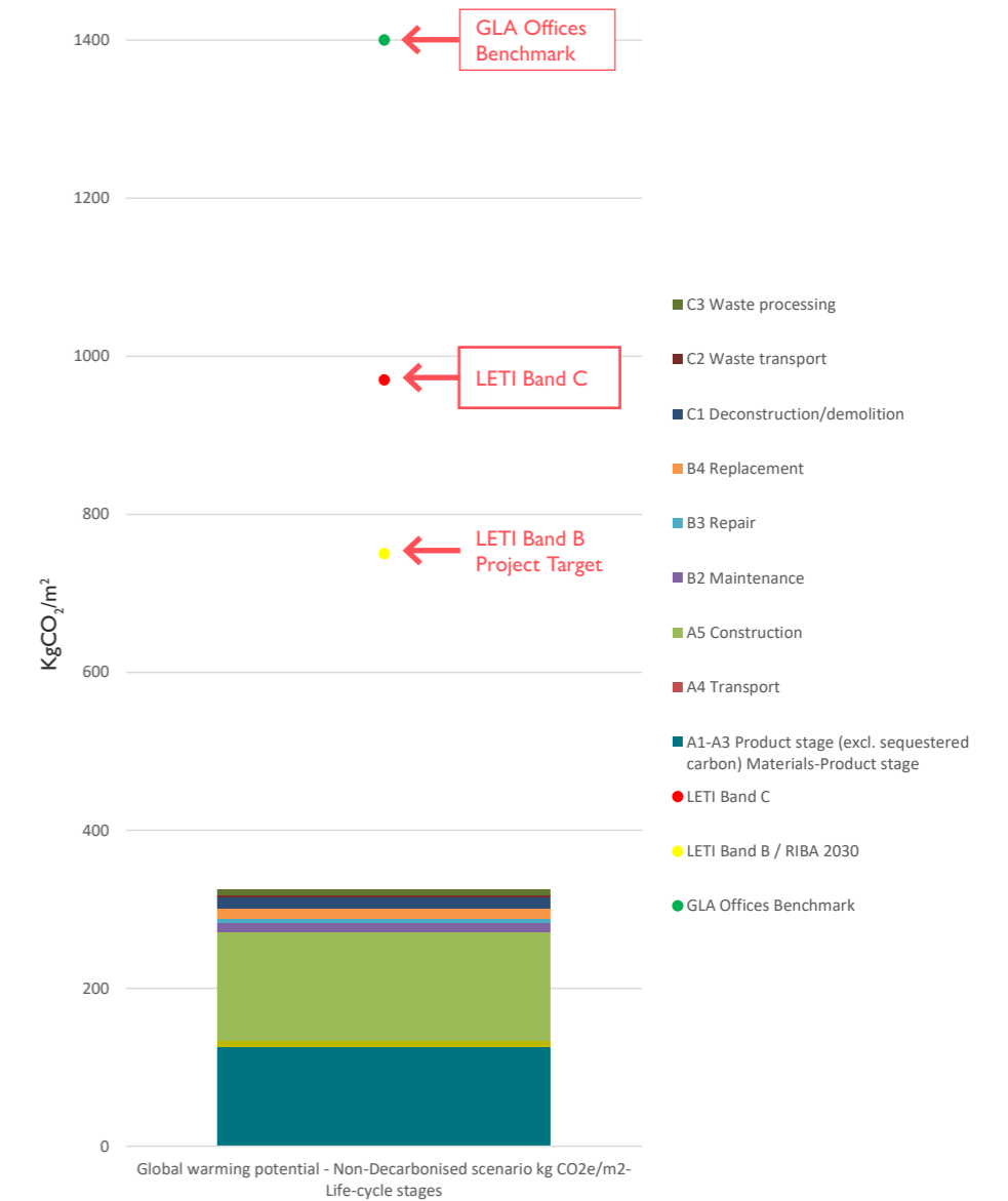
Global Warming Potential (Non-Decarbonised Scenario) Kg CO 2 e/m 2 (Stage A to C)
