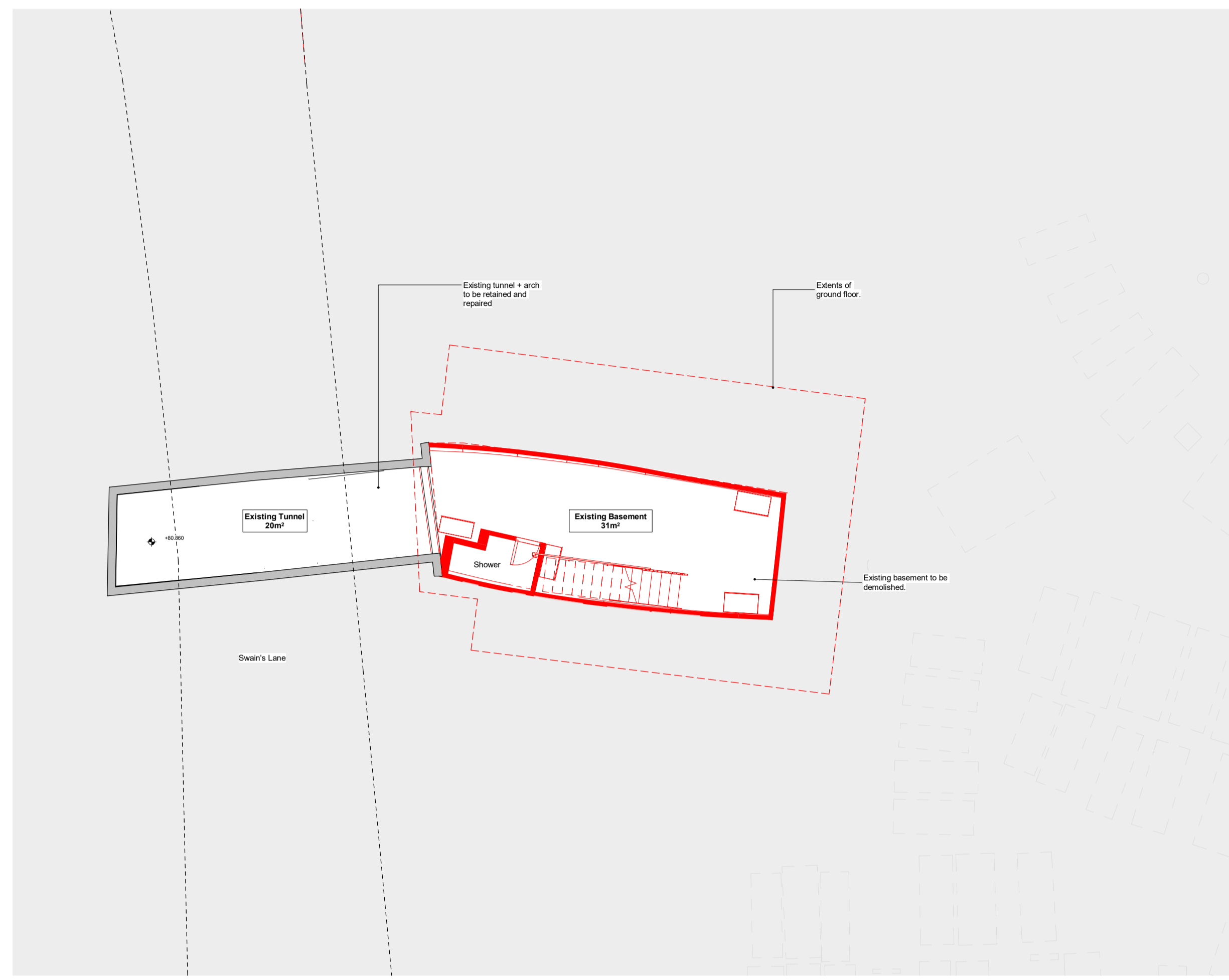
2 Basement - Existing East Lodge - Demolition Plan 1:100
