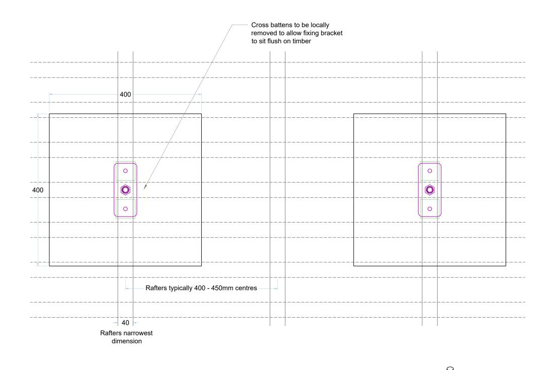
WEATHERING DETAIL 18mm pipe detail will allow collar to be fitted over 16mm stud
