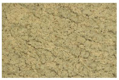
5687 Insoluble fines  $<63\mu m$  Stereomicroscope x20
