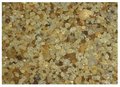
5687 Insolubles >63µm Stereomicroscope x10
