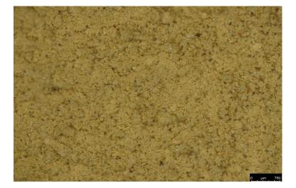
5530 Insolubles >63μm Stereomicroscope x10
