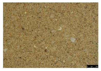
5531 Insolubles >63μm Stereomicroscope x10
