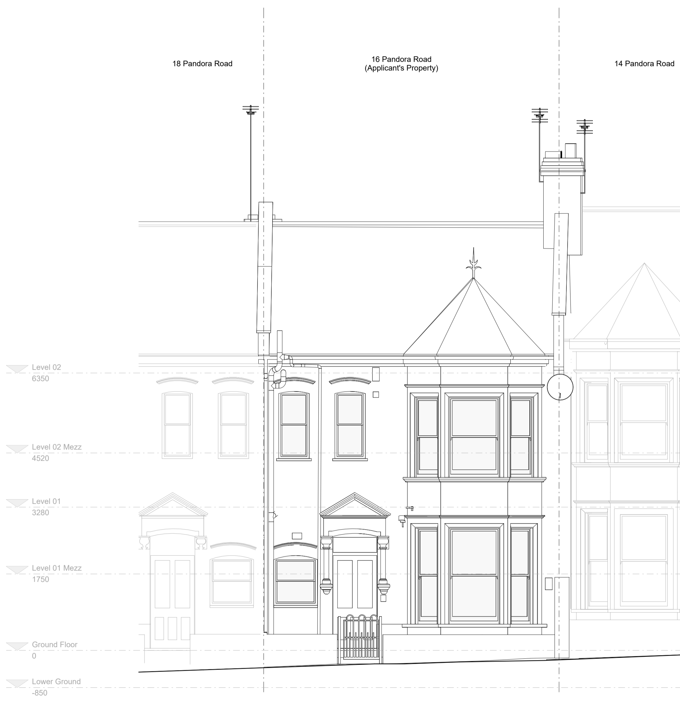
1 Existing - Front Elevation 1 : 50
