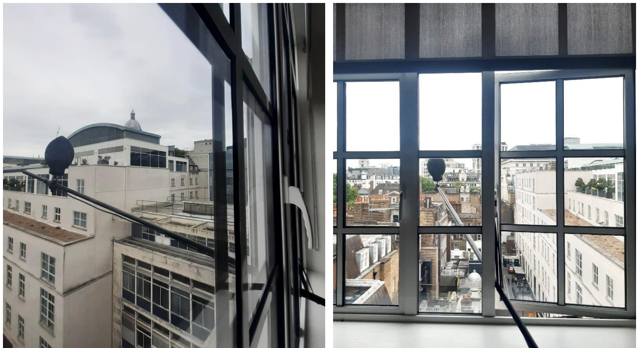
Figure 4 Sound level meter installed for unattended monitoring
