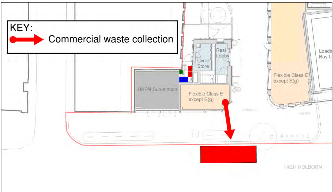
Figure 15 High Holborn commercial waste collection procedure
