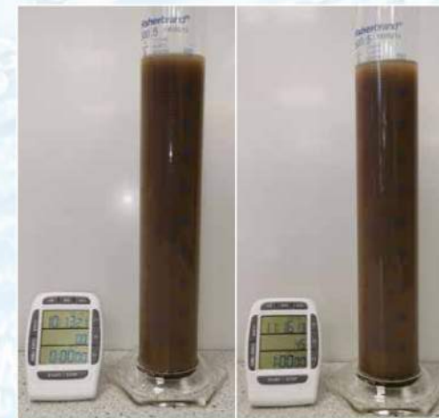
Settlement of clay particles from time 0-60 mins
