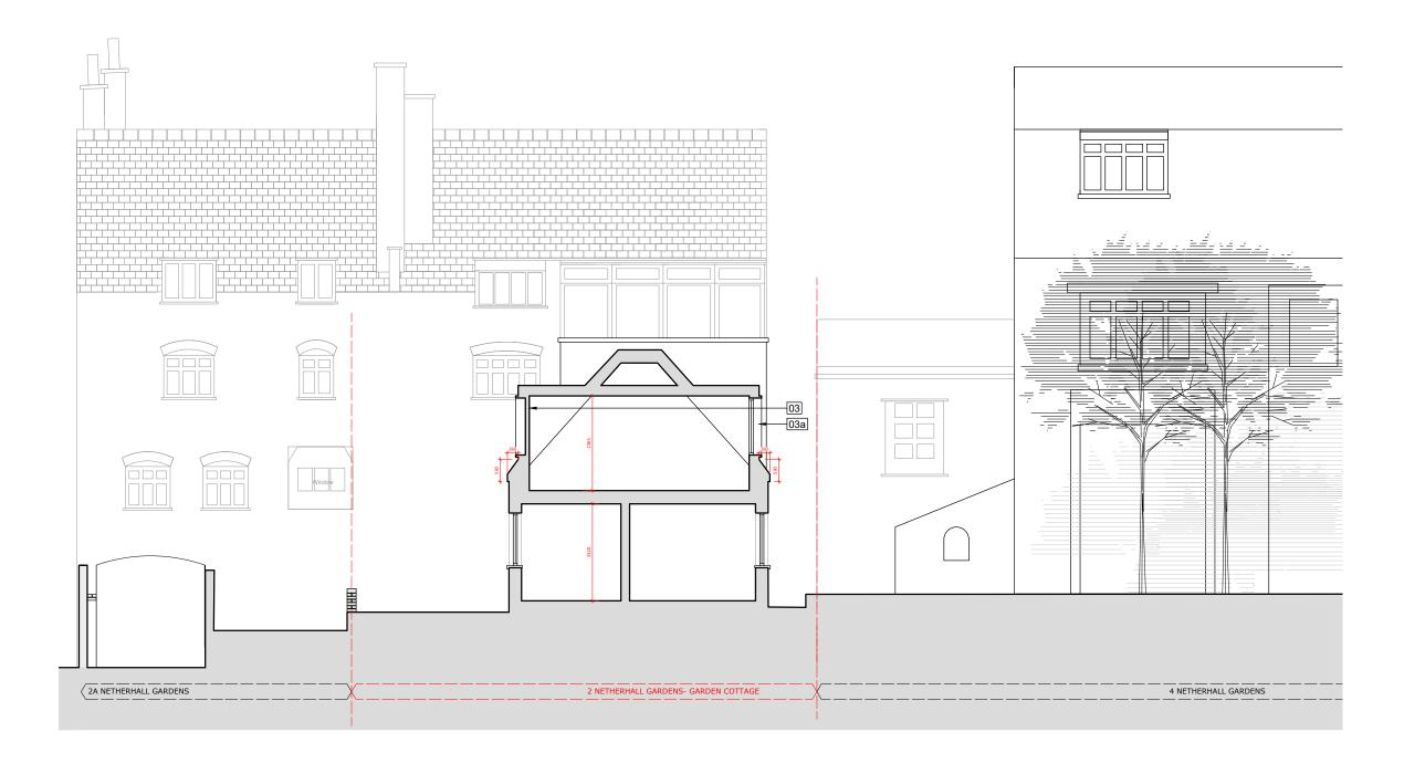
New blind dormer extensions in timber construction with zinc clad cheeks and a custom Accoya timber framed fixed insulated panel system with a vertically coffered design
