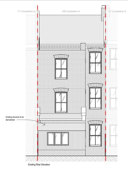
109 Constantine rd 07 Constantine rd conservation style Replace all existing rear windows with traditional wooden sash windows , colour and style to match existing. Replace all existing front windows with traditional wooden sash windows , colour and style to match existing. TITIT Proposed roof skylights sed side extension infill Proposed new rear structure with glazing design -SCAL DATE E 1:100 @A3 22/11/24 Proposed Rear Elevation
