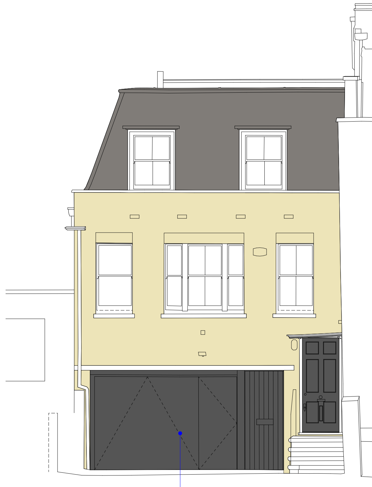
Existing Metal garage door with inset door
