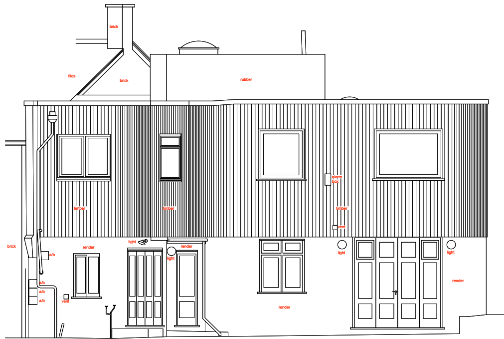
EXISTING NORTH WEST ELEVATION
