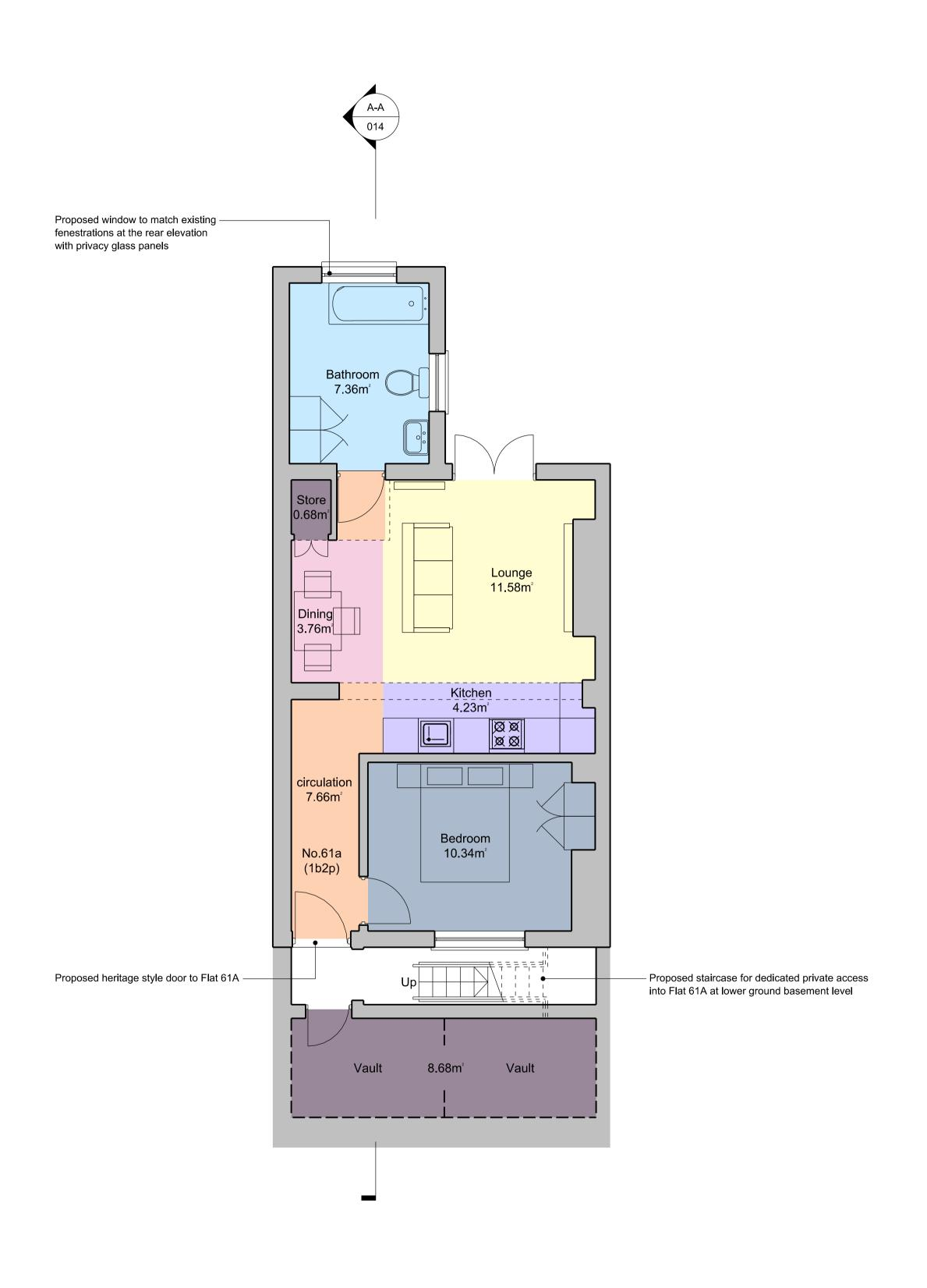
Proposed Lower Ground Floor Plan Scale 1:50 @A1 (1:100 @A3)
