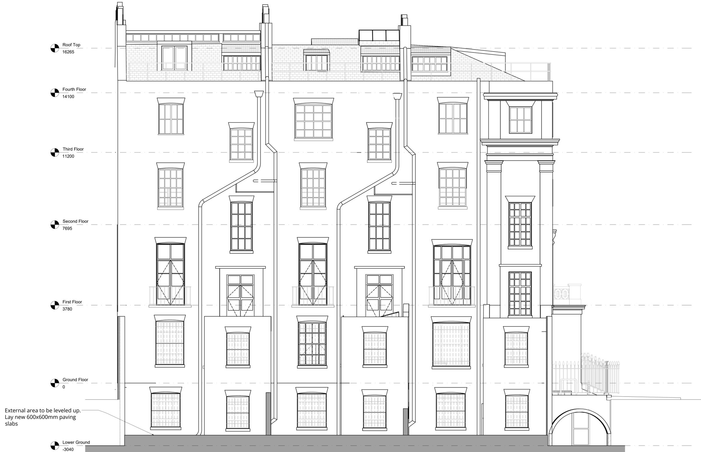
PROPOSED REAR ELEVATION (North-East Elevation)
