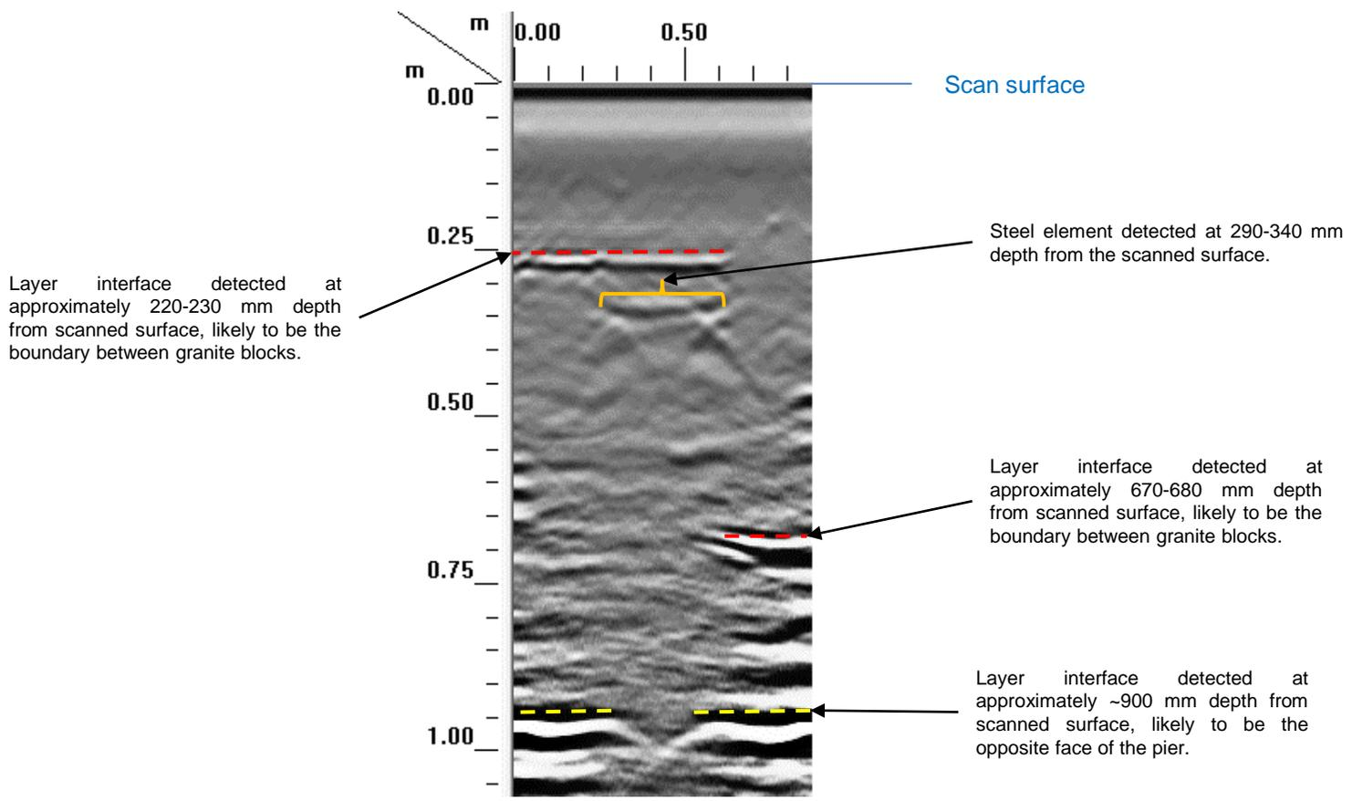
**Figure 1:** Typical radargram collected on the gate pier showing the features detected. All depths quoted are from the scanned surface.
