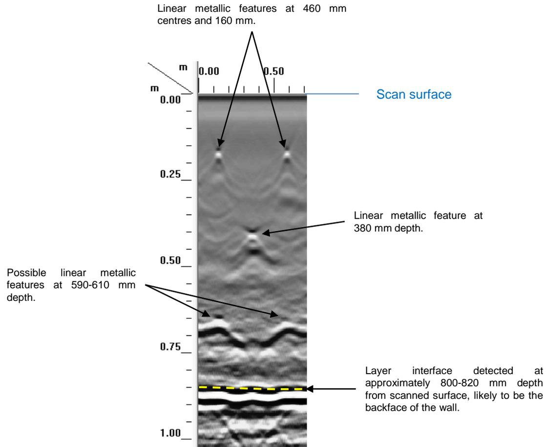
**Figure 2:** Typical radargram collected on the face of the granite support wall showing the features detected. All depths quoted are from the scanned surface.
