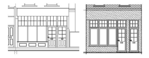
• The structure of the front wall is wrong – the front shop windows do not have a central column, yet one is shown.
