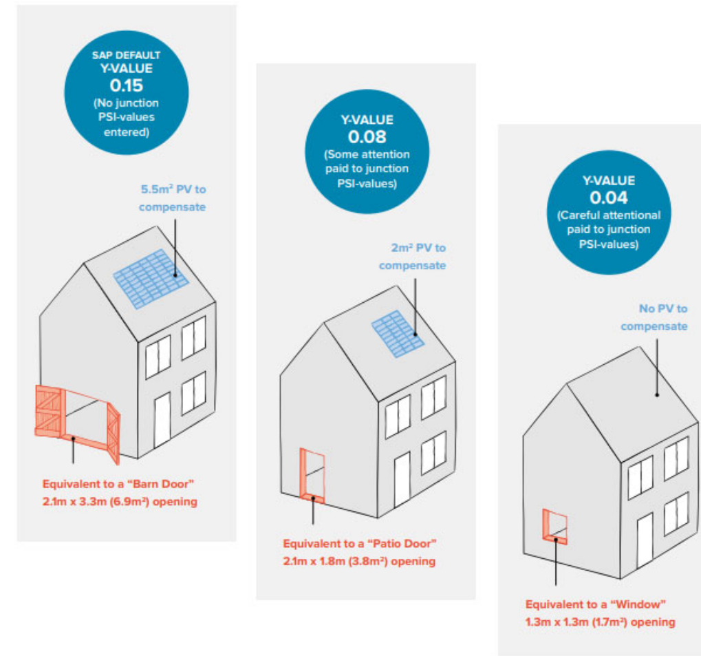
Figure 4.2.4.2 - Thermal Bridging Impact in SAP (Ref: Thermal Bridging Guide, Zero Carbon Hub)
