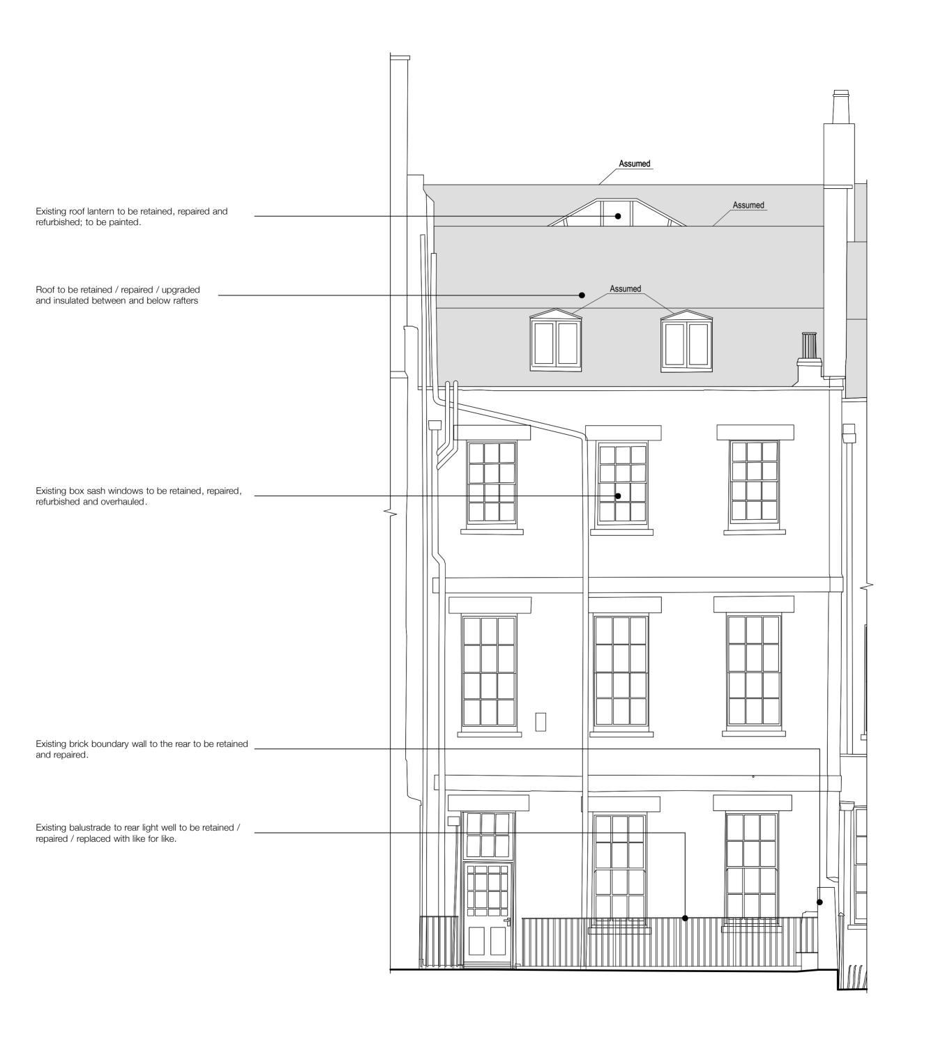
Indicative drawing based on and derived from Measured Survey Pro
