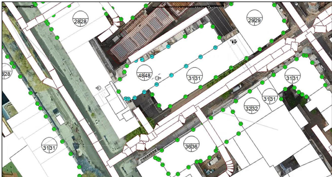
Figure 10 - Predicted noise levels with no acoustic treatment - Level 12 Plant
