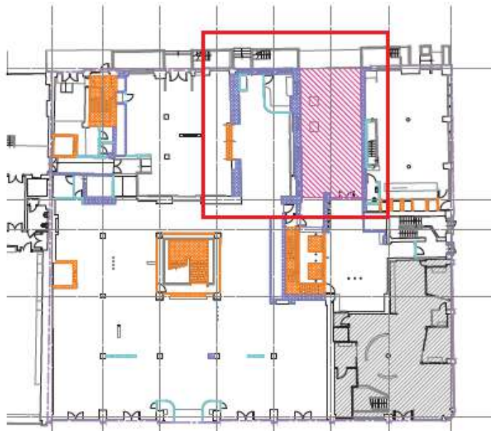
Figure 26: Proposed demolition at ground floor. Highlighted in red, the infill area proposed to be demolished. In orange, stairs, lift and shafts to be demolished.
