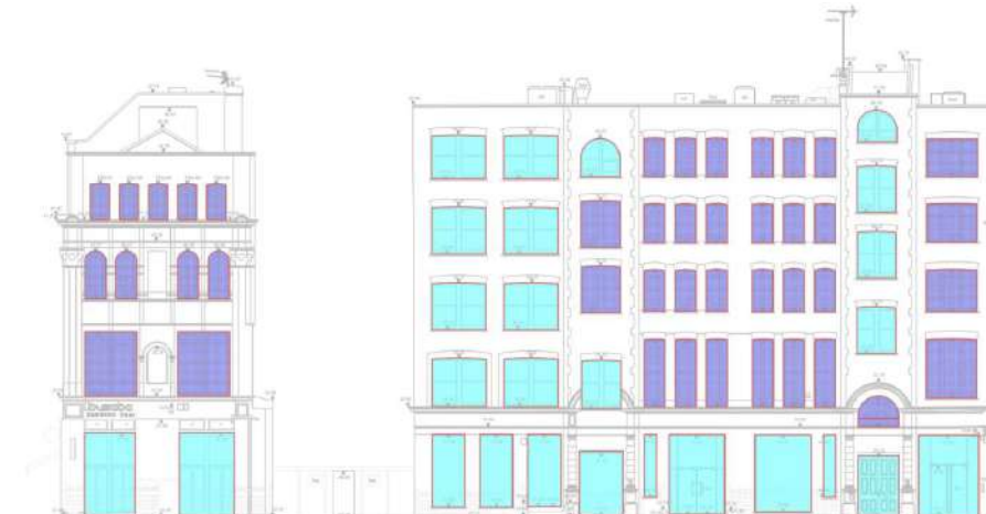
Figure 18: Demolished (blue) and retained (purple) glazing on Alfred Place
