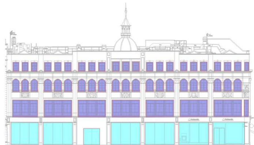
Figure 15: Demolished (blue) and retained (purple) glazing on Tottenham Court Road
