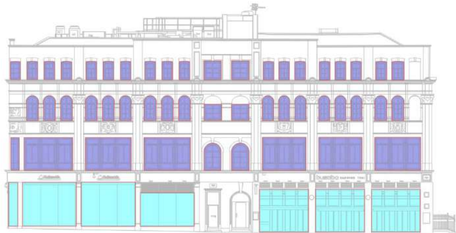
Figure 16: Demolished (blue) and retained (purple) glazing on Store Street
