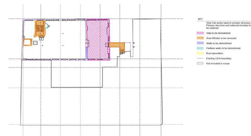
Figure 11.2.1: demolition drawing showing Building A retained at L04 (2311-EMR-Z00-004-DR-A-70206) and L04 of the Proposed Development (TCB-EMR-Z00-004-DR-A-02106) demonstrating minimal new office space construction.
