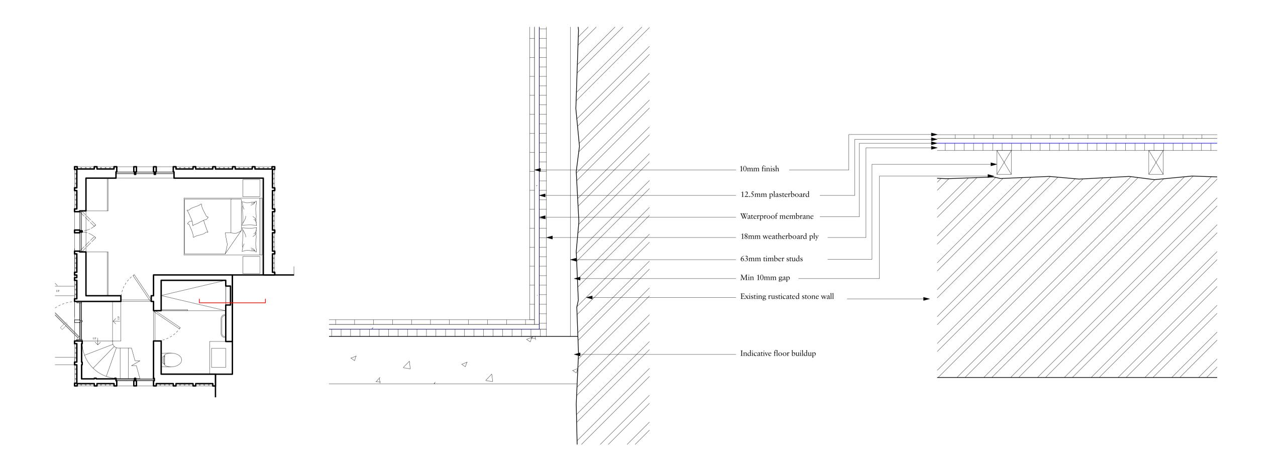
Preliminary Detail Section through Proposed Bathroom Shower Wall
