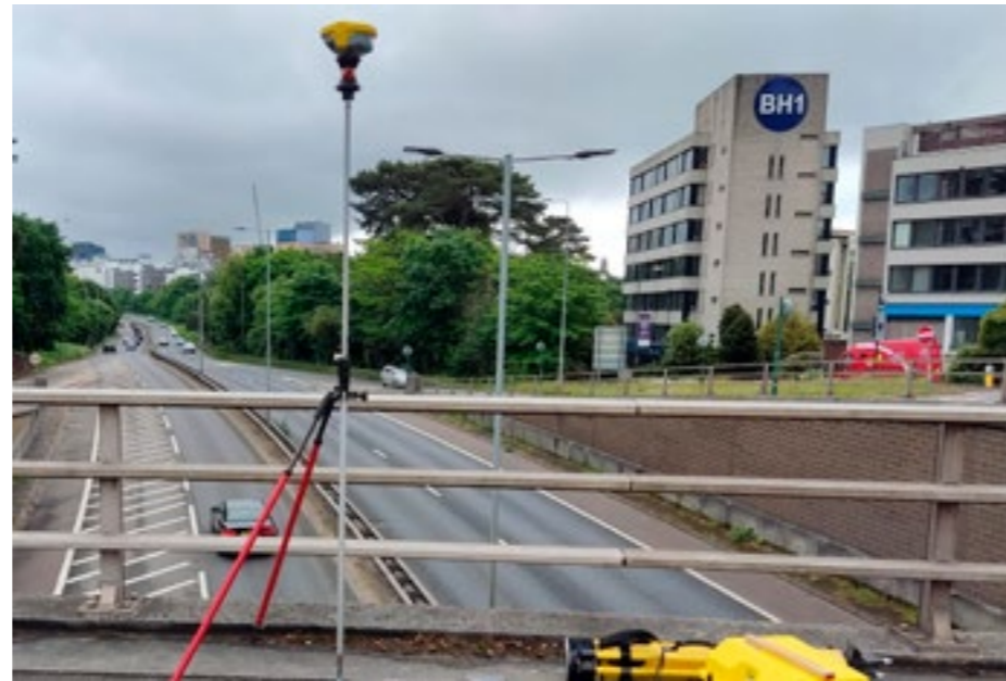
7: Field survey being carried out, GNSS receiver
