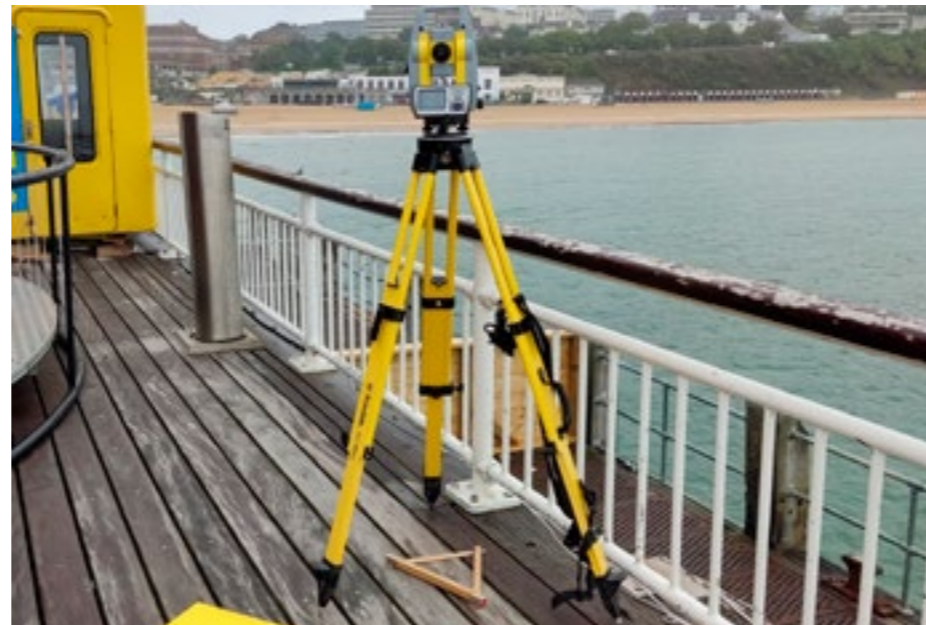
8: Field survey being carried out, total station
