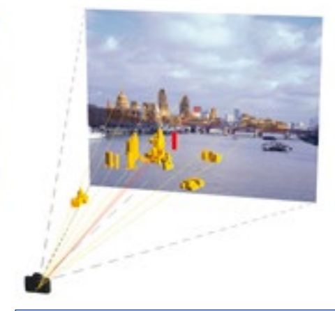
17: The camera matched background plate with an example of a proposed scheme included in red
